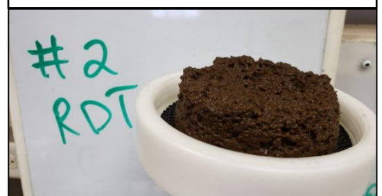
Figure 5 - Rapid dewatering test, retained solids
