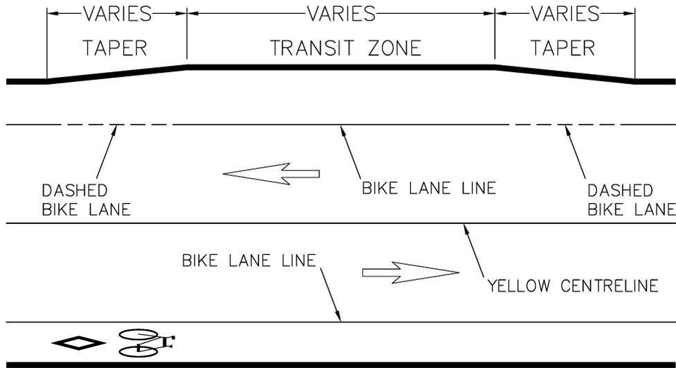
**Typical Paint Markings for Bicycle Lanes** Source: *Bikeway Traffic Control Guidelines for Canada*
