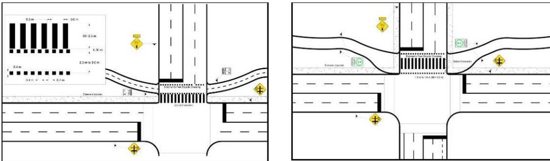
**Examples of Bicycle Pavement Markings at multi-use trail crossing (unsignalized intersection)** Source: *Bikeway Traffic Control Guidelines for Canada*
