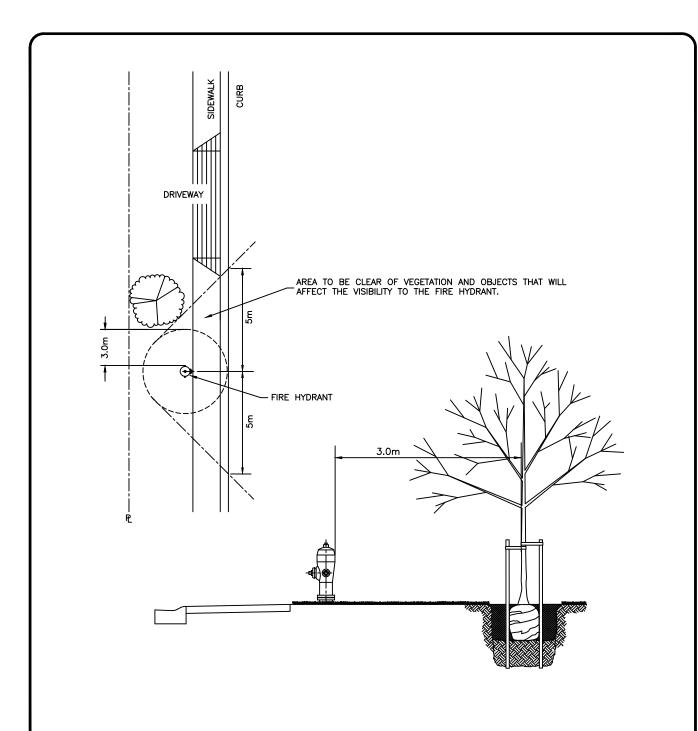
NOTE: TREES (AND ANY OBJECT OR BUILDING) NEED TO BE LOCATED, AT A MINIMUM, 3m FROM A FIRE HYDRANT. THERE SHOULD BE A MINIMUM OF 5.0m CLEARANCE, ON THE ROAD, IN FRONT OF A FIRE HYDRANT.
