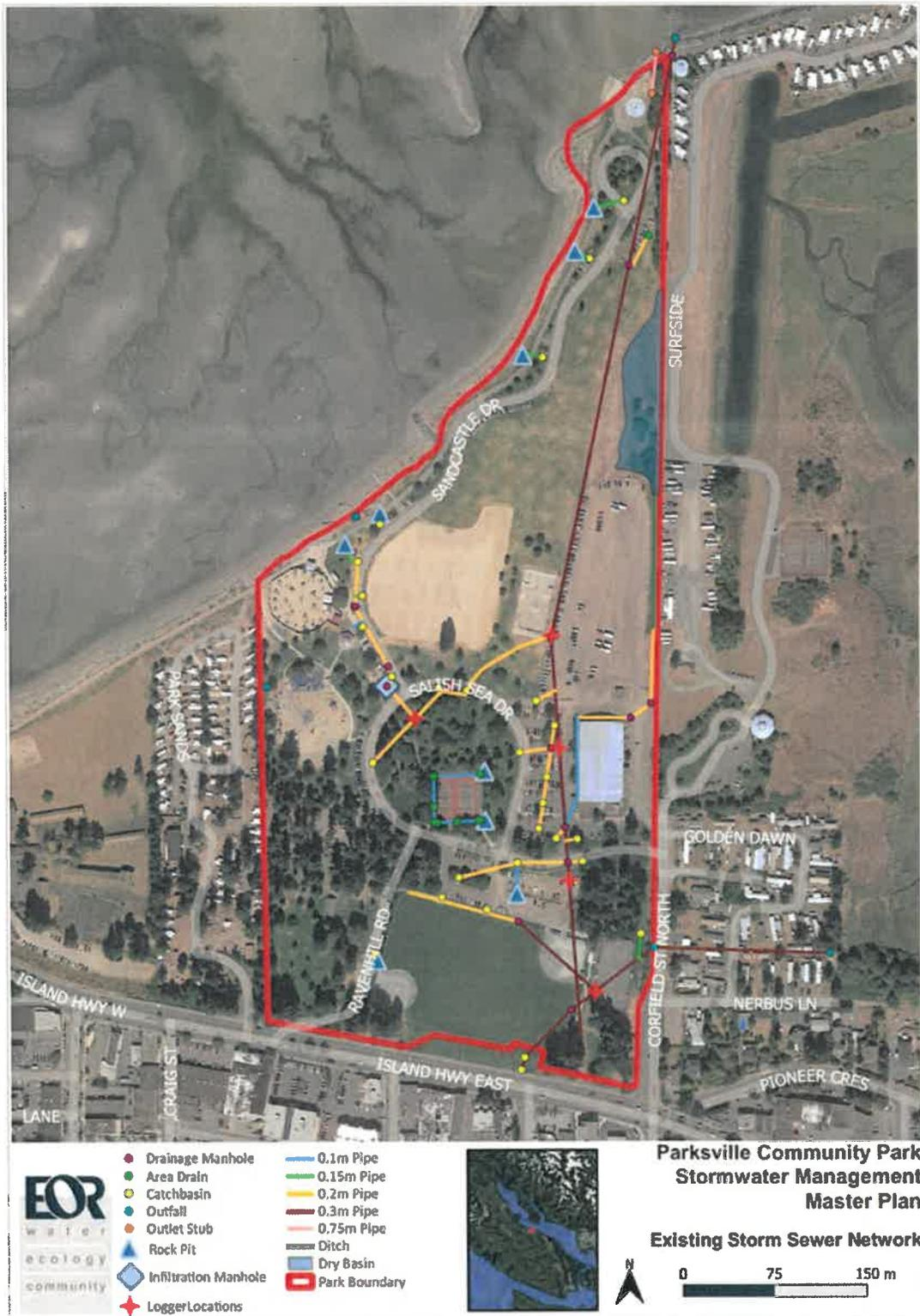
Figure 23. Existing Stormwater Management System
