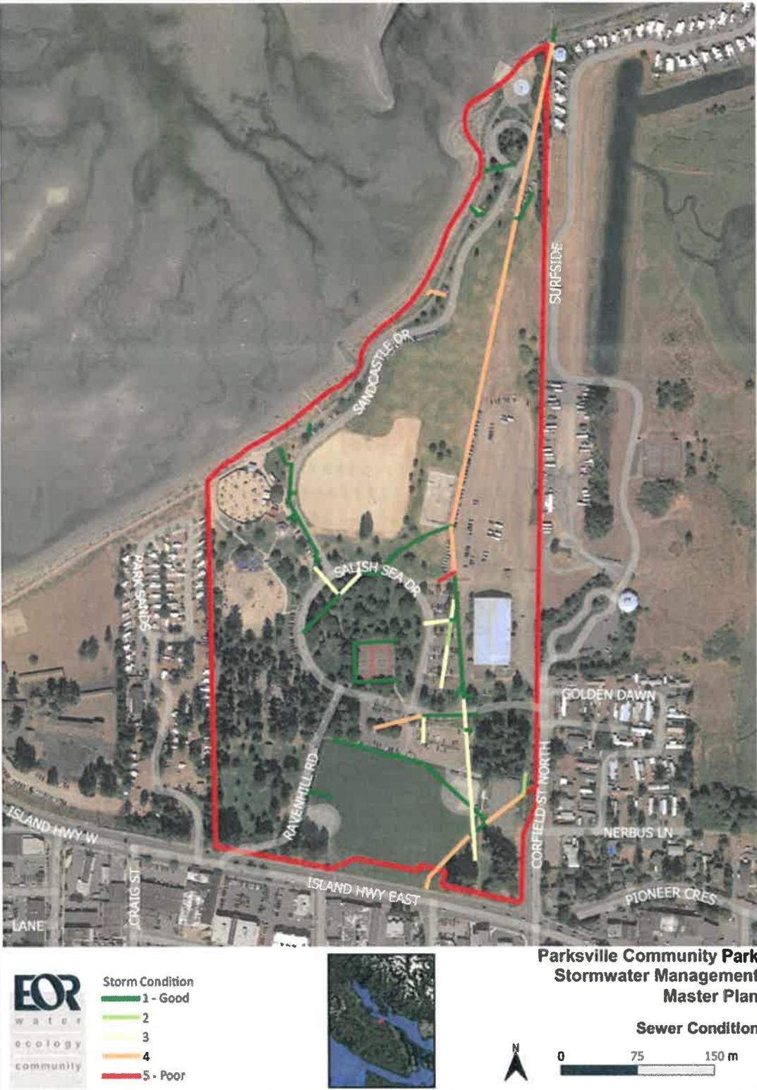
Figure 24. Estimated Sewer Condition
