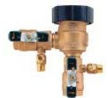
**Reduced Pressure Backflow Assembly (RPBA)** – An assembly containing two independently acting, internally loaded check valves separated by a reduced pressure zone. Used for severe hazard applications where an approved air gap is impractical.
