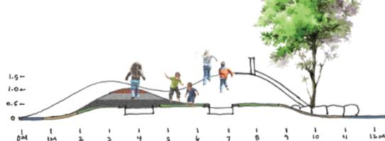
The tree planting zone will be ~4m diameter, with 1m deep soil, topped with engineered wood fiber.
